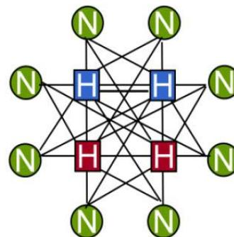
The speed of the fabric is only part of the story as ATCA has an advanced topology that allows for the potential doubling of the total system throughput.
