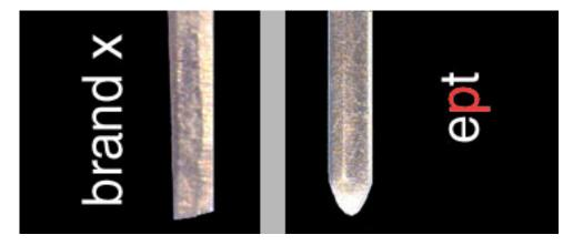
These microscopic pictures compare connector pins of a competitor and ept. The pin to the left shows the rough surfaces and burrs caused by stamping. The rolled ept pin on the right has much smoother surfaces. These differences explain the enhanced mating and contact qualities of the ept pins.
