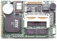
and a CompactFlash<sup>™</sup> solid state disk socket with two RS-232 serial ports, an IDE HDD interface, and a floppy disk controller, as well as one PCI-Bus subset interface for functional expansion.
