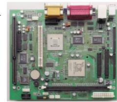
manufactured to consumer specifications. This includes increased resistance to vibration, shock, humidity, moisture and heat. The low power, fanless operation of the GX1-233 processor also enables reduced heat buildup in the chassis, helping to extend the MTBF of any system the board is applied to.
