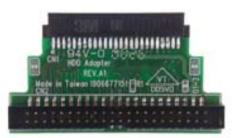
CompactFlash to HDD Adapter
