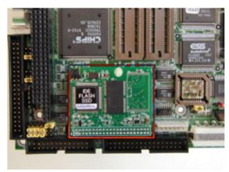
Advantech will begin to sell its new IDE interface Flash disk at the end of May this year. The PCD-1244H will be an effective replacement of our current PCD-1230A, which has already been phased out. The PCD-1244H will retain the same form factor and product characteristics as the PCD-1230A, but offer double the memory capacity. Three memory sizes of 8 MB, 16 MB and 32 MB will be offered. The increased memory capacity reflects the never ending effort by Advantech to pass on
