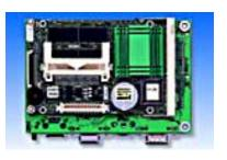
bi-directional printer port (which supports SPP, ECP, and EPP modes), an IDE HDD interface as well as one ISA interface for functional expansion. There is also a reserved 36-bit interface to add a CPC-2520 VGA/LCD module. Users can choose various functions that more closely fit their application needs.
