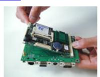
The much anticipated CPC-2420 is now available. This new tiny carrier board comes with a SODIMM socket for carrying the CPC-2245/N Mini Biscuit SBC and has standard I/O connectors such as VGA, LCD, LAN, FDD, IDE, serial ports and a printer port.
