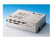
Advantech's MBPC-300 Series 5.25" Biscuit PC chassis and power supply support two new SBCs that add increased power, offer more features and provide greater flexibility to this PC chassis line. The PCM-9570 and PCM-5864/L SBCs help round-out this chassis line and give all-in-one solutions that Advantech customers need. The MBPC-300 has always been an ideal case for system integrators implementing applications that include Wallmount PC controllers, Embedded PC controllers,
