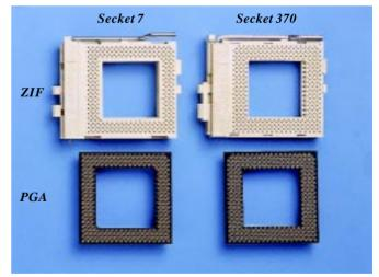
ZIF/PGA type Socket 7 & Socket 370
