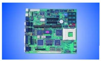
POS-460 Rev.B1 486-based POS Control Board
