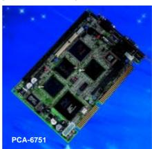
Pentium® MMX CPU is mounted directly on board, with a frequency choice of either 166 MHz or 266 MHz. Mounting CPUs directly on-board eases the configuration and installation
